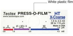
Remove the Testex Tape from the surface and place the replica between the anvils of the Testex Gauge, making sure that it is centred properly.
