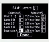
Record the pass/fail result and the nature of fracture - cohesive, adhesive, and glue failures - using the app (left) or the instrument's touch screen display (above)
