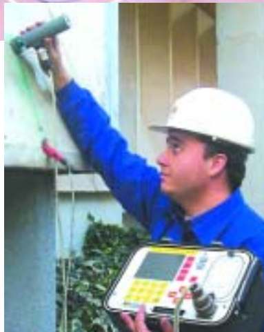
Sensor "C" for Very Wet Submerged Structures
