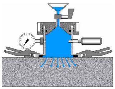
maintained by means of a micrometer gauge pushing a piston into the chamber. The piston movement compensates for the volume of water penetrating into the material.
