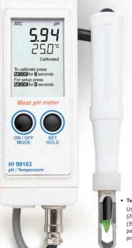
Two blade lengths available Use the optional FC 098 (20 mm) or the included FC 099 (35 mm) stainless steel meat penetration blades for meat processing applications
